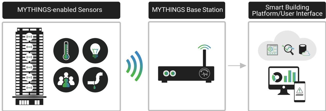
**The MYTHINGS Architecture:** MYTHINGS-enabled sensors wirelessly transmit data to a MYTHINGS Base Station, equipped with MYTHINGS Central for network and device management. Data is then pushed to the users preferred backend/cloud for analytics and visualization.
